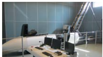
EJECTION SEAT SIMULATOR Repeatable, realistic ejections in a controlled and safe environment. Computer-based ejection decision making scenarios.
