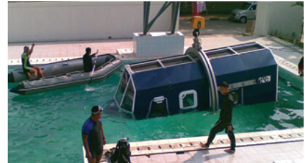
WATER SURVIVAL TRAINING A turn-key system of trainers that teaches water survival training skills for aircrew. Trainers include Helicopter Rescue Hoist Trainer, Underwater Escape Survival Trainer, Parachute Drag Trainer and Parachute Drop and Disentanglement Trainer.
