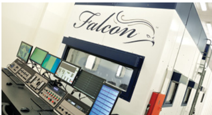
FALCON HYPOBARIC (ALTITUDE) CHAMBER Supports high altitude exposure training and is designed to perform up to 100,000 feet. Chambers available in various sizes.
