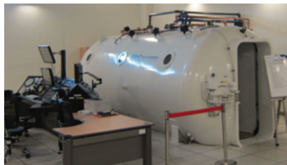
MULTIPLACE HYPERBARIC CHAMBER Station chamber designed to provide hyperbaric oxygen therapy. Chambers are available in various sizes.
