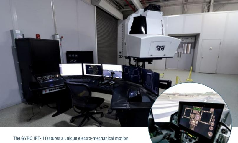
The GYRO IPT-II features a unique electro-mechanical motion base with generic or aircraft specific cockpit configuration, creating a realistic flight simulation environment.
