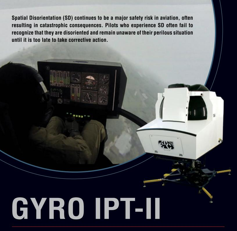
Training in a customized motion simulator helps pilots recognize the early signs of SD and be able to take corrective actions to regain orientation and evade a mishap.
