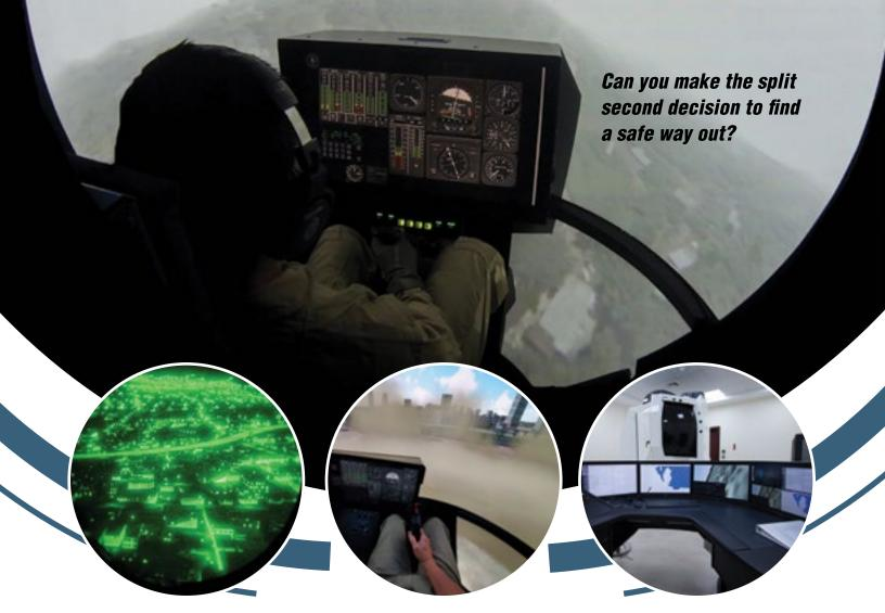
The GAT-HELO is a full-motion SD Simulator that realistically reproduces the Degraded Visual Environment (DVE) and SD situations during flight simulation. It features a generic light helicopter cockpit with interactive flight controls, realistic computer-generated instruments and a dome visual display providing an immersive flight experience.
